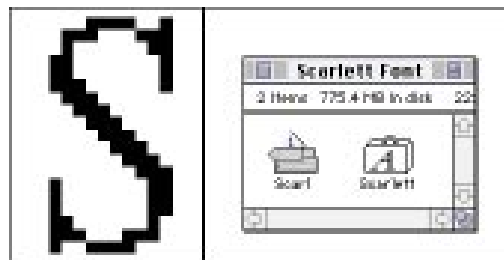
figure 1 / Plagued by the jaggies? For those running ATM, the jagged look might be caused by not having both parts of a PostScript font (right) installed.
