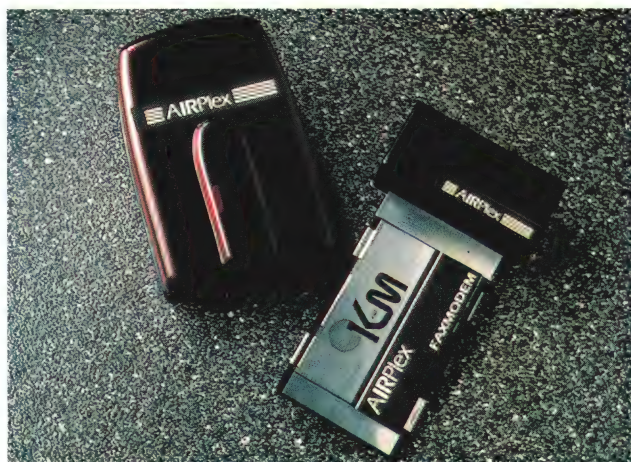
THE AIRPLEX CORDLESS FAX-MODEM uses an infrared signal to send data from a notebook to a receiver attached to the phone jack.
