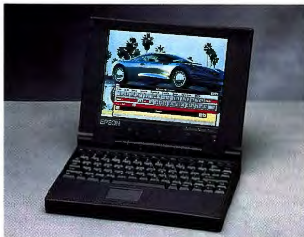
FINGER-POINTING IS ALLOWED WITH EPSON'S ACTIONNOTE, one of the first portables to integrate Synaptics' TouchPad pointer.
