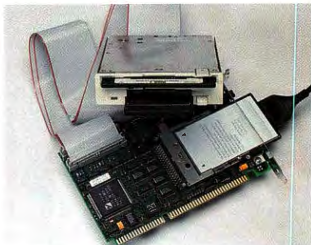
THE SCM SWAPBOX CLASSIC COMBO and Premium Combo both pack a PCMCIA slot and a floppy drive in a 3½-inch drive bay.
