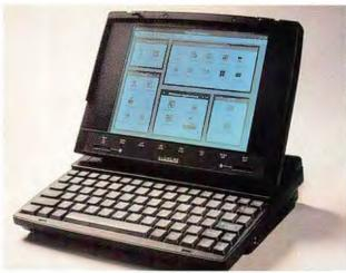
An optional coprocessor encrypts all your files inside the SLOO7 20-MHz 386SL notebook, which features 4MB of RAM, a 60MB hard drive, and a 10-inch backlit VGA screen.
