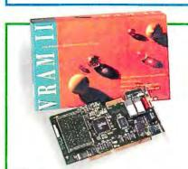
Video 7 ... 7 years 9768 VRAM II VGA 1 MB—Fast, flicker-free high performance 16-bit VGA. Uses dual ported RAM for optimum performance. Ideal for Windows, CAD/CAM/CAE, OS/2 and other graphics intensive applications . . \$329.
