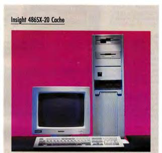
The Insight 20-MHz 486SX includes 4MB RAM, 64K RAM cache, a 130MB IDE hard drive, two floppies, a 14-inch super-VGA monitor, and 16-bit super-VGA card—all for \$1995.
