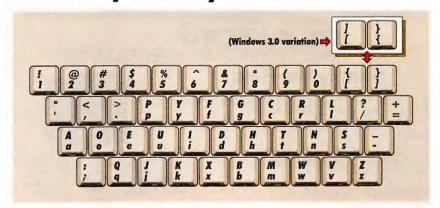
FIGURE 1: The Dvorak keyboard layout is designed to let you type as fast as possible. Photocopy this chart and use it for reference while learning to touch-type with the Dvorak layout.
