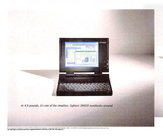
serial and parallel ports, a Super VGA CRT port, a mouse port, and an optional internal modem or fax modem. Not to mention an optional external battery slice for a total of over five hours of power. All of which permits it to perform feats far beyond the reach of ordinary notebooks, far from home.
