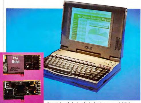
A panel above the keyboard is the door to easy upgradability for notebooks in the VIP M line from ALR, allowing you to step up to 486 processors.
