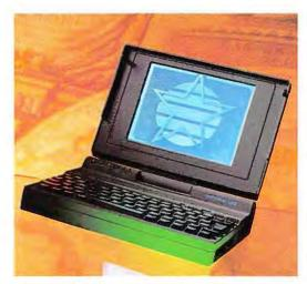
Light and airy at 8.3 pounds traveling weight, the LSX will keep cooking for over 5 hours with power saving turned on.
