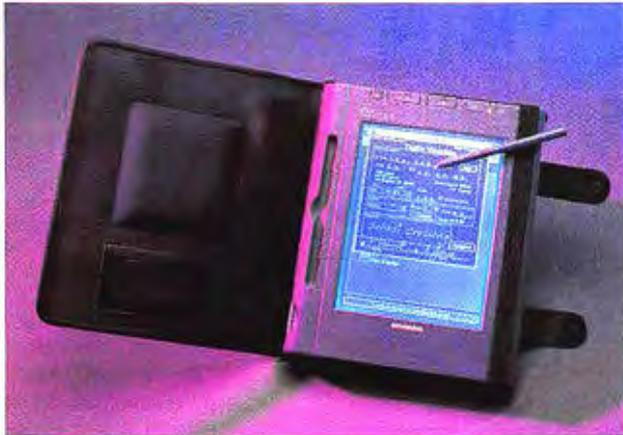
Samsung's PenMaster is a 386SL tablet-style pen computer that weighs less than 5 pounds and runs up to 3 hours.
