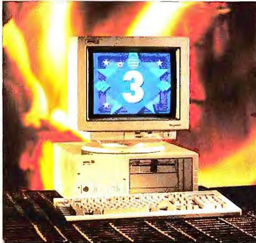
The well-made 2386E puts everything up front, including the power switch, reset button, and keyboard port.
