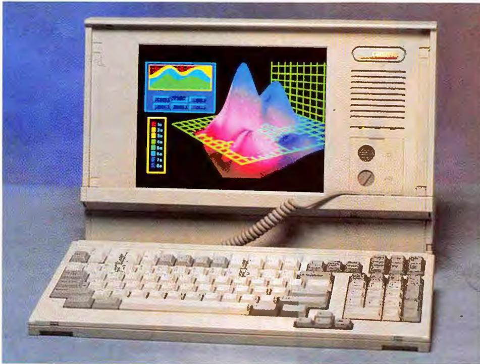
Offering 486 power and an active-matrix color screen that's better than a standard desktop VGA monitor, Compaq's Portable 486c weighs in at almost 18 pounds.
