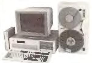
Now you can exchange data files between your IBM PC/XT/AT and any mainframe or mini-computer using IBM compatible 1600 or 6250 BPI 9-Track tape. Unit can also be used for disk backup. Transfer rate is up to 4 megabytes per minute on PCs and compatibles. Subsystems include 7" or 10½" streaming tape drive, tape coupler card, cables and software.
