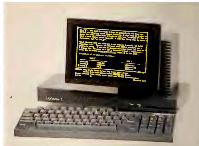
Emerald's sleek Lanstation I, with a built-in electroluminescent display and a 20MB hard disk option (but no floppy), offers LAN data security.
