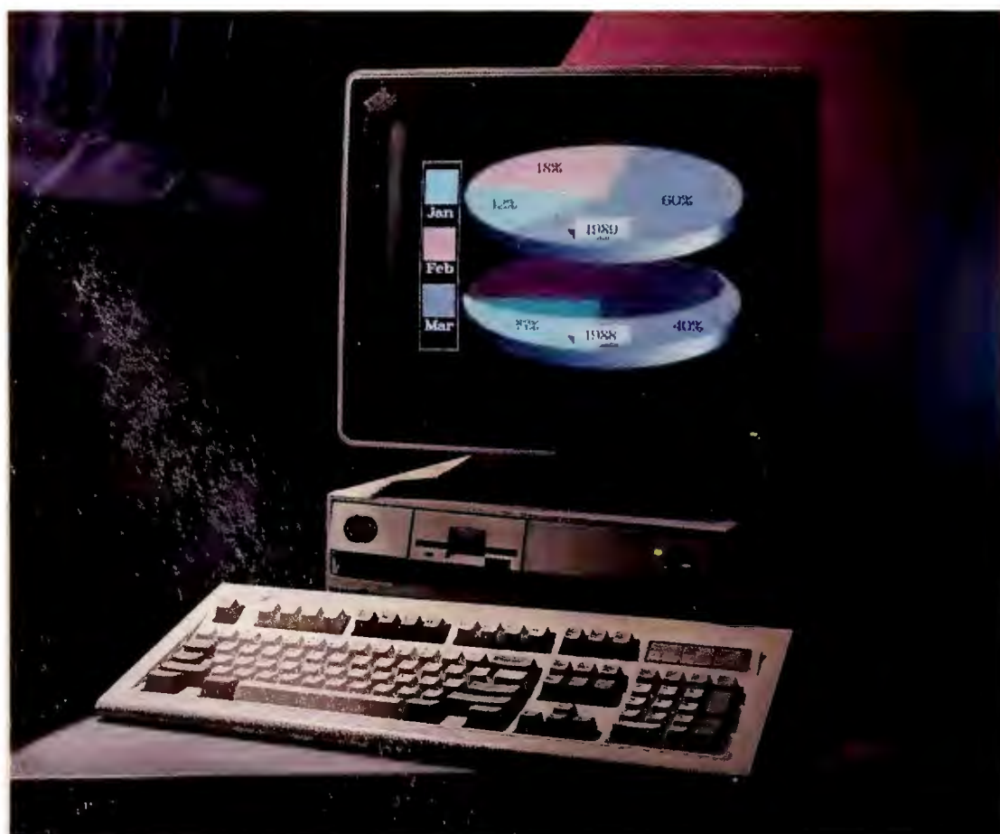
IBM's unit has the highest price and the lowest capacity for fast RAM. The PS/2 Model 70 486 is also the slowest DOS unit—but, surprisingly, the fastest 486-based OS/2 machine.
