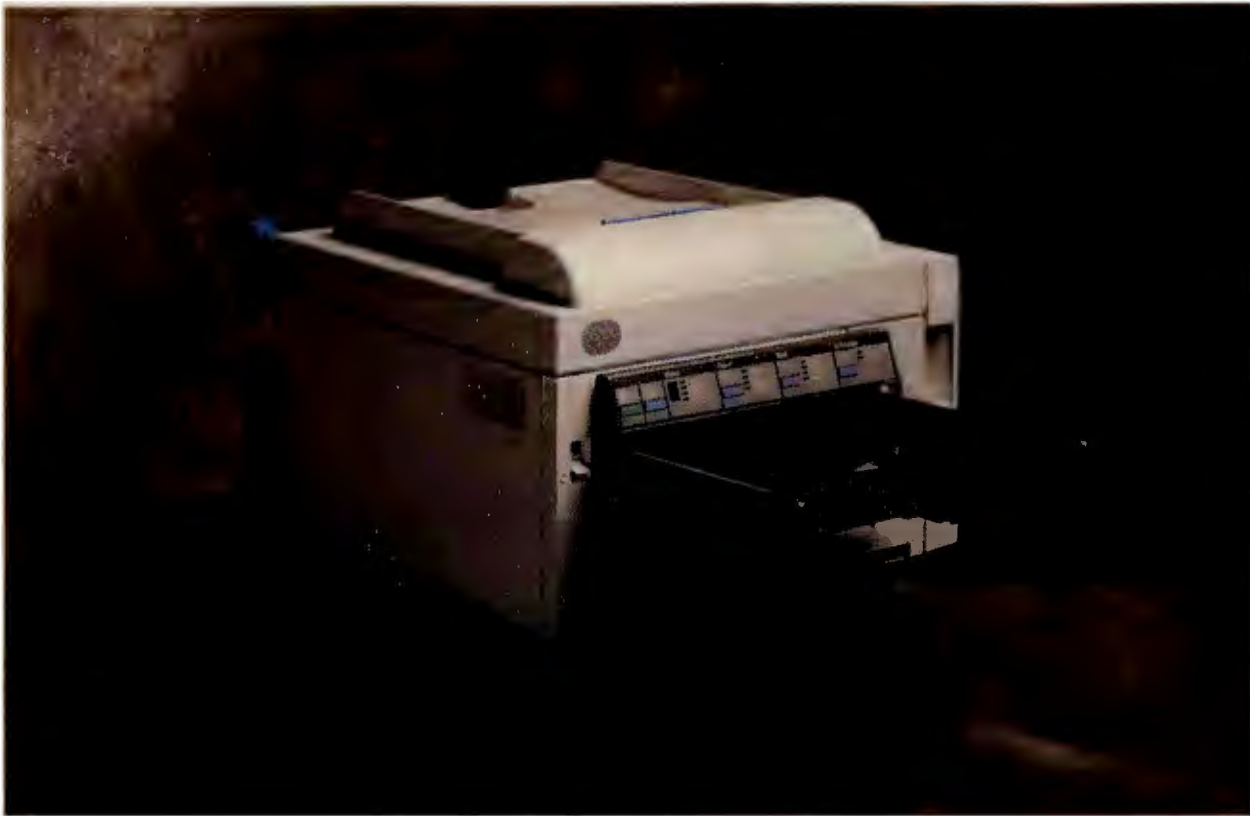
The LaserPrinter E, an inexpensive addition to IBM's LaserJet-compatible line, brings 5-page-per-minute performance and upgrade options into the contest with Hewlett-Packard's LaserJet IIP.
