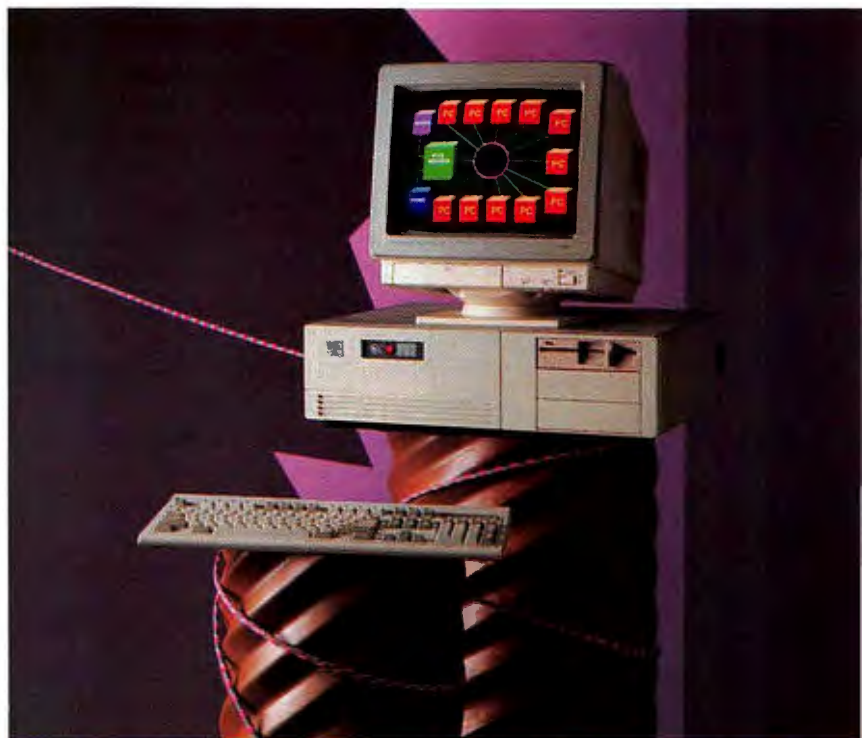
The second-fastest system in the roundup, the Micro Express ME 386-25 goes for an incredibly low $6325—with 4MB RAM, 150MB ESDI hard disk, and monitor, no less.
