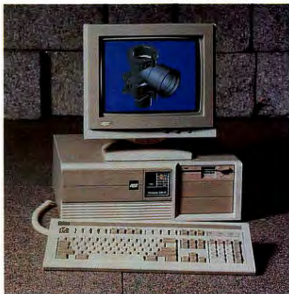
The sleek AST Premium 386/33 holds its CPU, cache controller, and memory cache on a removable board, while offering CPU-speed access to 36MB of 32-bit memory. The base configuration costs $6965.
