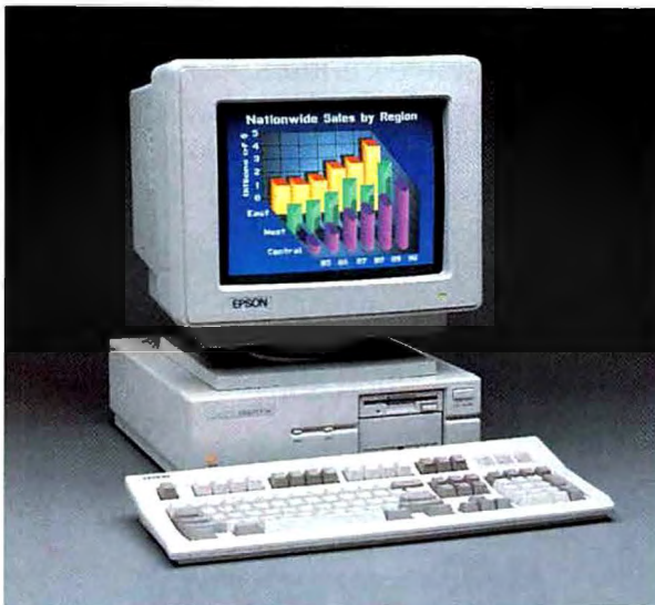
Epson's new IBM PS/2 Model 30 clone, the Equity Ie , brings a 25 percent faster processor and an additional 8-bit expansion slot to the party. The small-footprint unit includes MCGA graphics on the motherboard.
