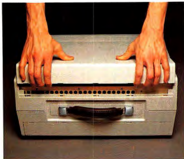
Figure 1: The insides of the COMPAQ are accessed by prying off the side panel on the case
