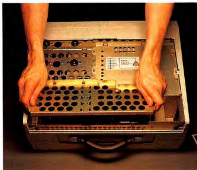
Figure 2: Removal of the system-board retaining cover
