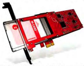
CETON'S DIGITAL CABLE Quad-Tuner Card is a PCI Express card that lets you record up to four shows at once, including premium channels.
