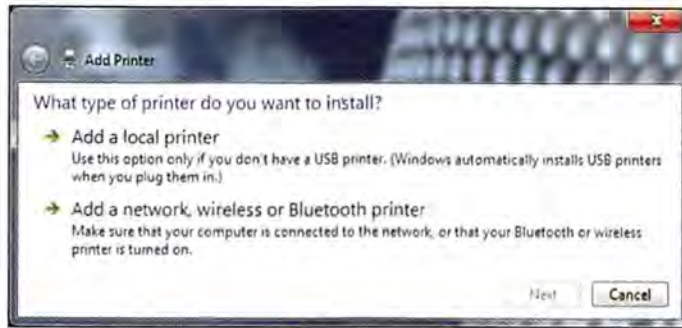
CLICK THE SECOND button in Add Printer to step through the wizard screens.
