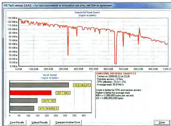
AS THIS HARD-DRIVE benchmark indicates, the maximum read speed for files drawn off our networked hard drive is 95.8 megabytes per second.
