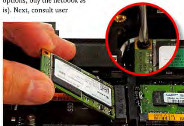
ON A DELL Mini 9 netbook, the solid-state drive is easy to find near the other components. It's a small card held in place by two screws.
