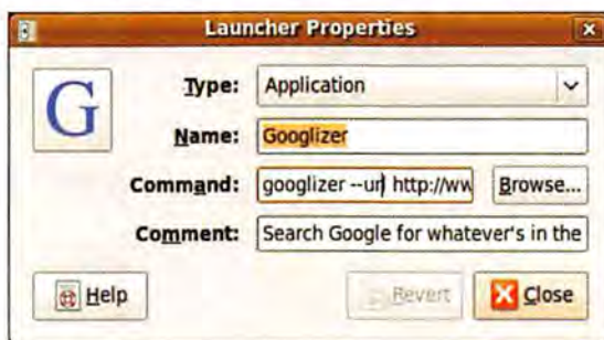
WITH A SIMPLE change of the URL in the Command field, you can turn the Googlizer search applet into a dictionary tool.
