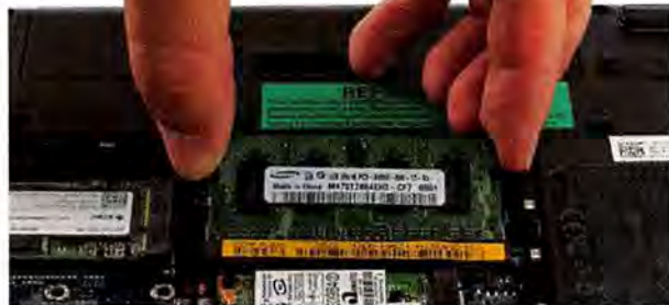
LIKE ORDINARY LAPTOP RAM, netbook RAM is easy to replace once you remove the main cover plate on the bottom of the machine.
