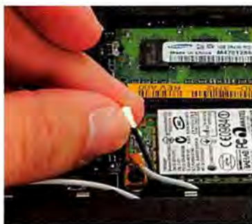
TO UPGRADE YOUR netbook's Wi-Fi card, begin by disconnecting the two antenna cables from the card.
