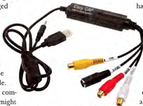
YOU CAN CONNECT your old videotape player to a simple, affordable USB converter such as the EasyCap to digitize your old video—and audio, too.
