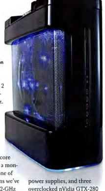
overclocked nVidia GTX-280 graphics boards are completely submerged in nonconductive oil. Though its configurations start at about \$4500, the Reactor we tested broke the \$10K barrier with three 64GB solid-state drives (in RAID 0) for your boot volume, plus two 1-terabyte 7200-rpm drives (mirrored in RAID 1) for file storage. Total hard drive space that's actu-
