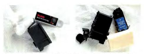
KODAK'S INK CARTRIDGE (left) holds a large wad of cotton, whereas the G&G Products ink cartridge uses a piece of foam rubber. In our tests we extracted all of the ink from these materials and from the ink wells.
