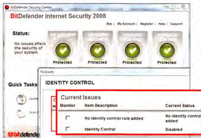
BITDEFENDER'S INTERFACE NEEDS a little work; it reports a status of 'Protected' when its Identity Control feature is actually disabled.
