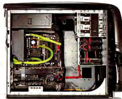
KEEPING IT COOL: Alienware's Area-51 7500 uses a silent liquid-cooling system (the green pipes shown) to temper its overclocked processor.
