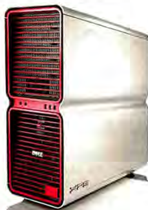
DELL'S STYLISH XPS 720 includes Intel's newer QX6800 CPU, overclocked to 3.2 GHz.
