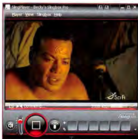
HOME-MEDIA BOXES SUCH as Slingbox require upload speeds of 600 kbps; 1 mbps to 2 mbps is recommended.
