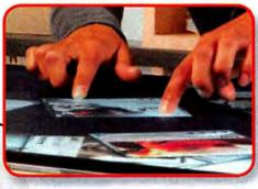
SURFACE WILL RECOGNIZE up to 52 points of touch at any one time, thanks to five cameras within the table that are trained on overlapping sections of the top. As with Apple's iPhone, you can use two fingers to stretch or shrink a photo. You can also rotate a shot, toss it to the side, or stack it with others.
