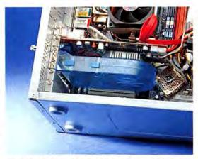
FIGURE 3: KEEP YOUR GRAPHICS CARD cool with a fan designed specifically for it, such as Antec's \$20 VCool.
