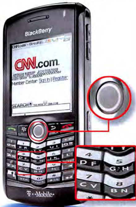
THE BLACKBERRY PEARL supports trackball menu navigation (upper left); its SureType system combines two letters on most keys (lower left). The microSD slot (right) is inconveniently located behind the battery.
