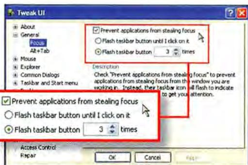
**FIGURE 1: USE TWEAK UI to prevent apps from jumping in front without first asking permission.**
