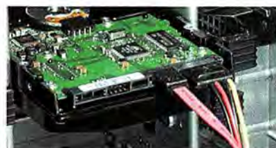
FIGURE 6: ATTACH the Serial ATA cable from the motherboard to the hard drive.
