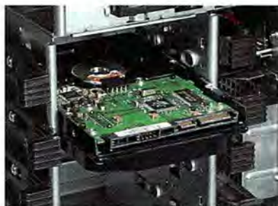
FIGURE 4: SLIDE the hard drive into one of the 3.5-inch bays until it clicks into place.
