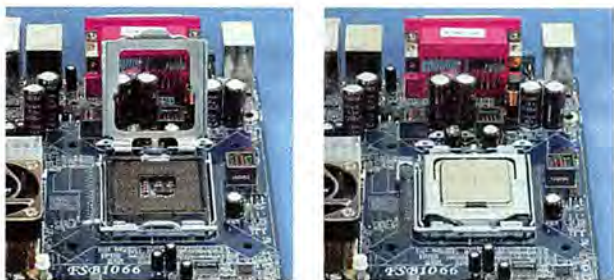
FIGURE 2: PLACE the processor in the motherboard's LGA socket and secure it by lowering the load lever over the top of the CPU.
