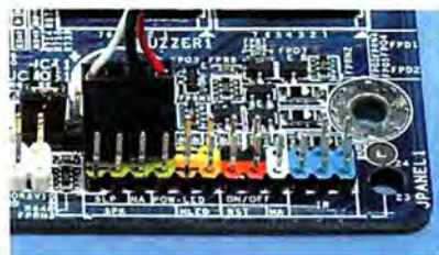
FIGURE 5: CONNECT the LEDs on the front of the case to their motherboard switches.
