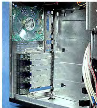
FIGURE 1: REMOVE the motherboard tray and I/O shield prior to installing components.
