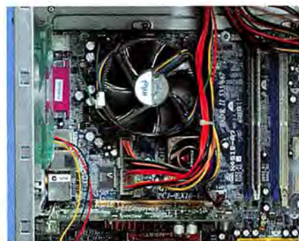
FIGURE 7: KEEP the air flowing through your case by tying off cables away from components.
