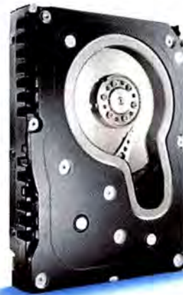
WESTERN DIGITAL'S Raptor X offers a window into its internal workings, and 10,000-rpm speed.
