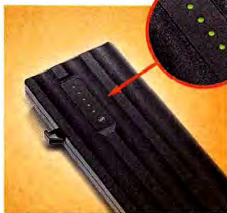
SOME BATTERIES, such as this one from a Dell laptop, are designed with an exterior battery meter.
