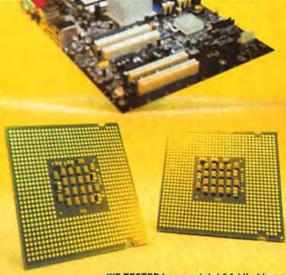
WE TESTED two new Intel 64-bit chips: a 3.6-GHz Pentium 4 and a 3.73-GHz P4 Extreme Edition.
