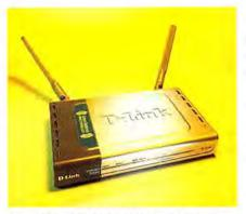
D-LINK'S SUPER G with MIMO router has two internal and two external antennas.
