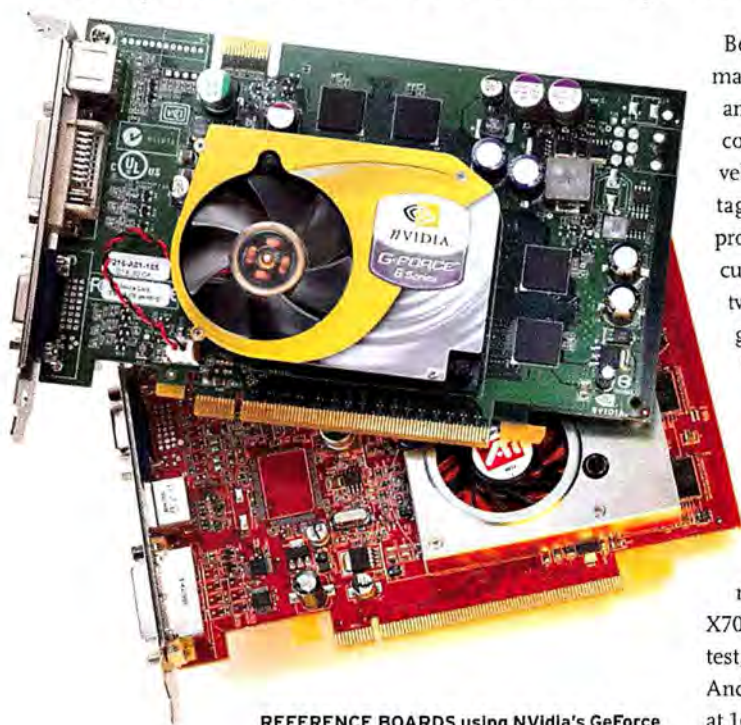
REFERENCE BOARDS using NVidia's GeForce 6600 GT (top), and ATI's Radeon X700 XT.
