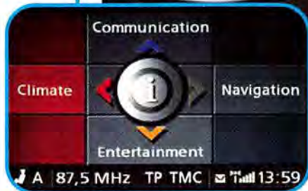
BMW'S 5 SERIES sedans sport its iDrive technology, featuring a joystick-style knob and menu button (above) that initiates a screen on the dashboard (left).
