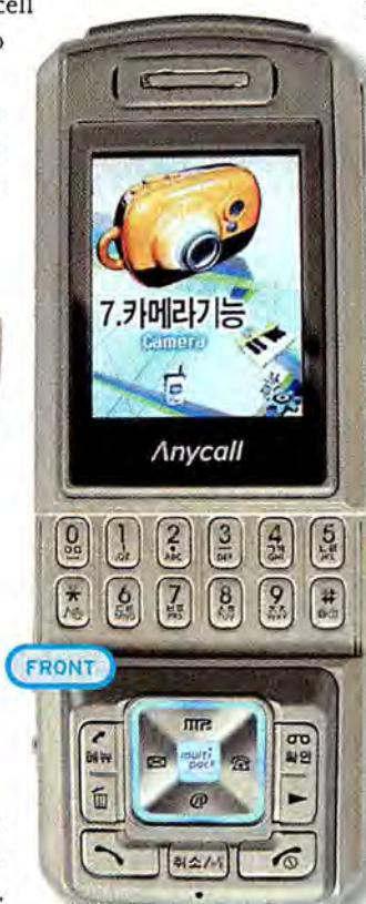
SAMSUNG'S SPH-S2300 cell phone sports a 3.2-megapixel camera.
