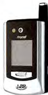
THE SAMSUNG SPH-V5400 has a 1.5GB hard drive.
