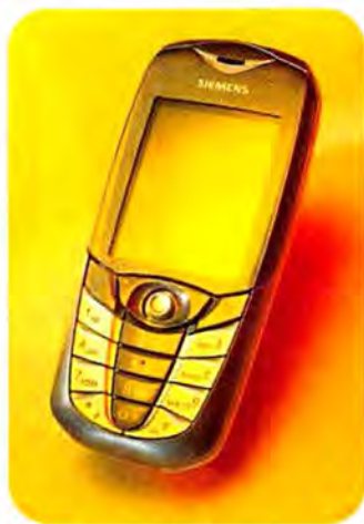
SIEMENS'S CX66 has a tiny joystick that is intended to make playing games easier.
