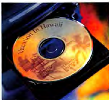
DOUBLE-DUTY LASER in a LightScribe burners cuts the disc labels and data.
