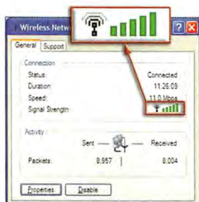
FIGURE 2: CHECK YOUR WIRELESS signal strength via your adapter's status utility.
