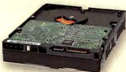
WESTERN DIGITAL'S Raptor WD360GD is the first 10,000-rpm Serial ATA hard drive. It's fast, but (at 36GB) too small for our chart.
