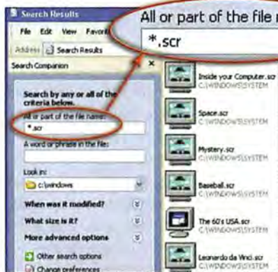
FIGURE 3: FIND AND DELETE unwanted screen savers by searching for all .scr files.
