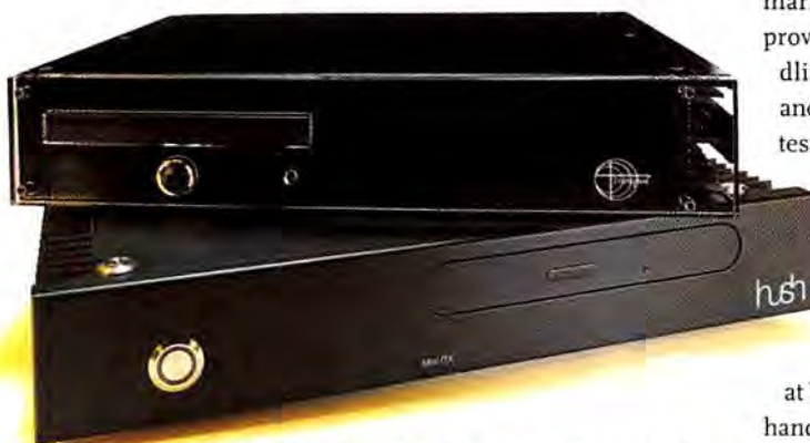
BOTH THE TRANQUIL PC (top) and the Hush Mini-ITX use fanless cooling technologies that let them run almost silently.
