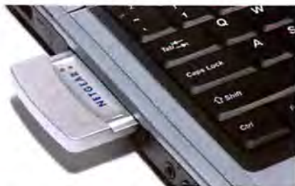
ADDING WIRELESS CONNECTIVITY to a notebook is simple: Install the wireless PC Card's driver, reboot, and insert the card in the laptop's PC Card slot.
