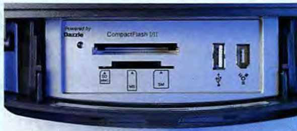
ONE SLOT ON THE HP Pavilion 775e reads CompactFlash cards, and another reads SmartMedia, SD, and Memory Stick.
