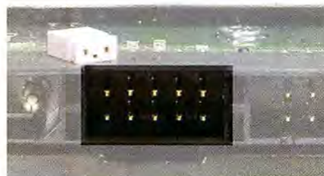
THE JUMPER PLUG fits over and connects two pins to designate a master or slave configuration; check your hard-drive manual for the proper settings.
