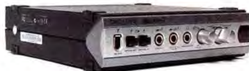
A FEW SOUND CARDS , such as Creative's Sound Blaster Audigy 2 Platinum EX, occupy two PCI slots—one for audio and the other for a joystick/MIDI port. The Platinum EX also comes with an external box for audio control and input ports.
