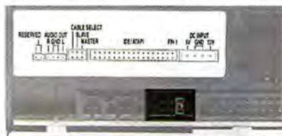
SOME OPTICAL DRIVES come with a handy, illustrated guide that shows you how to set the master/slave pins properly.
