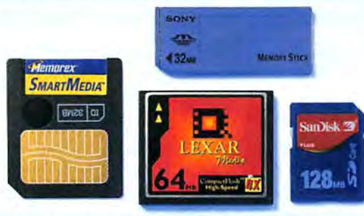
YOU CAN STORE OODLES of data on these cards; some CompactFlash cards are capable of holding 2GB worth of information.
