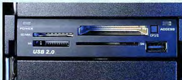
THE AMAX POWER P4 has four separate, dedicated card readers for CompactFlash, SmartMedia, SD, and Memory Stick.
