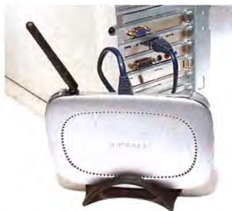
CONFIGURING A WIRELESS ROUTER such as NetGear's WGR614 involves connecting to a PC (via ethernet or Wi-Fi) and a broadband modem.
