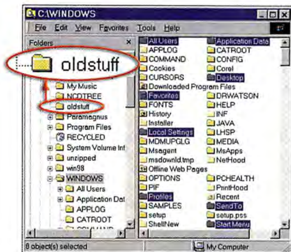
FIGURE 1: MOVE THESE FOLDERS from your Windows folder to 'oldstuff' prior to your OS reinstallation.
