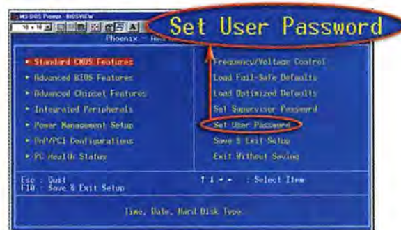
FIGURE 1: TO SET YOUR BOOT-UP PASSWORD , select this or a similar option on your PC Setup program's main menu.
