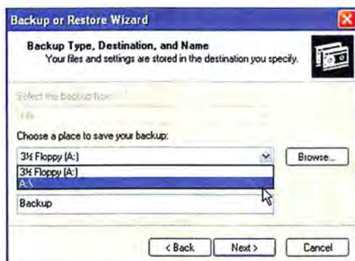
FIGURE 1: WINDOWS' BACKUP function works fine with most media but does not offer support for DVD.
