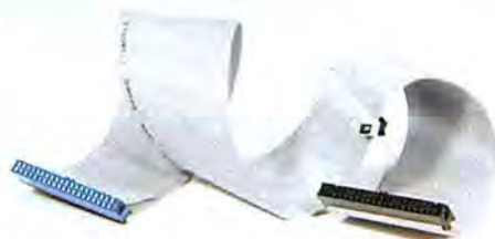
A PARALLEL ATA cable has three connectors: One end connects to the master drive, the middle to the slave drive, and the blue end to the motherboard.
