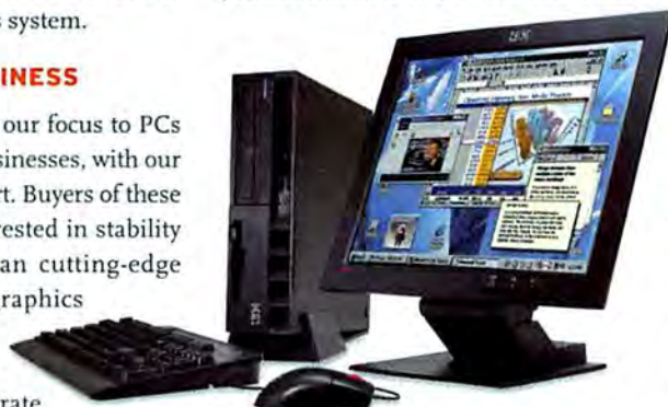
IBM'S NEW THINKCENTER S50 allows all components to be removed without tools.
