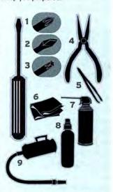
vents, revives blinded optical drives (see "Optical Drive Dilemma" on the previous page), and improves data connections. Electrical contact cleaner solution (8) cuts through grime and corrosion to improve electrical conductivity-just the thing for cleaning an old device. A handheld vacuum (9) lets you suck dust and pet hair out of less-accessible places.
