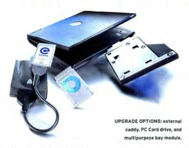
ON MANY LAPTOPS, replacing the 2.5-inch drive involves nothing more than unscrewing a panel, sliding the old drive out, and popping the new one in. Of course, you also need to transfer the data from your old drive-and that can be a challenge because most notebooks have space for only a single hard drive.
