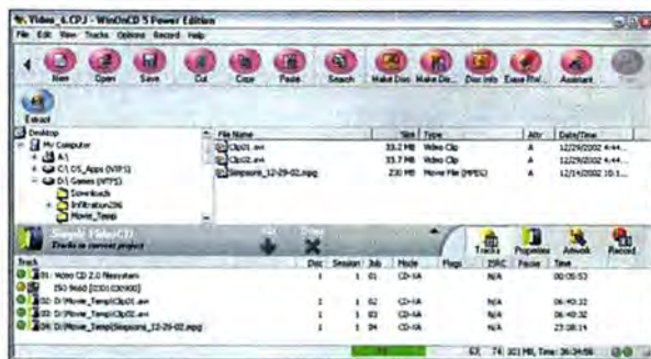
A SIMPLE VIDEO CD PROJECT in CeQuadrat's WinOnCD 5 Power Edition. WinOnCD re-encoded the two .avi files before burning.
