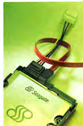
SERIAL ATA drives offer faster throughput and slimmer cables.
