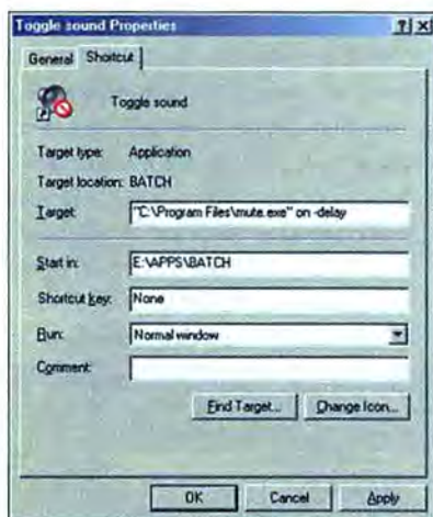
FIGURE 1: ENSURE A SILENT start-up by adding the on and -delay switches to the command line of the Mute freeware program.
