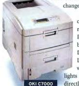
Oki Data's Okicolor C7000 series and the Xerox Phaser 1235 (both built around Oki Data engines) use LED technology in which an array of lights focuses an image
