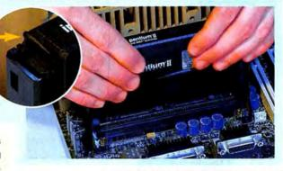
2 Insert the new processor module. Remove the new processor from its packaging, and gently slide it into the frame (it is designed to line up in only one way) until the cartridge is just above the slot. Then p
