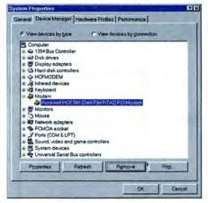
FIGURE 4: WHEN WINDOWS won't forget, uninstall old hardware drivers via Device Manager.
