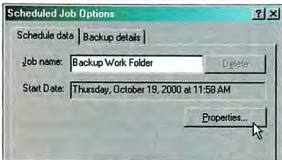
FIGURE 3: BACKUP SCHEDULING comes built into Windows 2000. Click Properties to specify schedule options.
