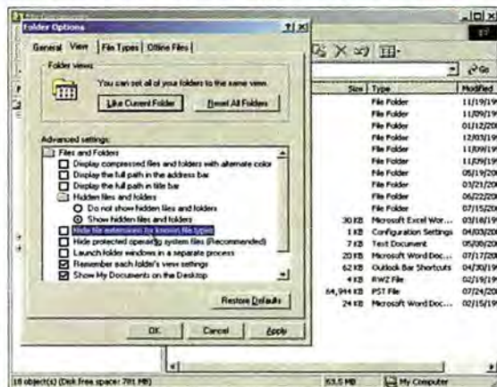
FIGURE 1: TO EXPOSE E-MAIL VIRUSES masquerading as innocent file types, uncheck Explorer's 'hide' option.
