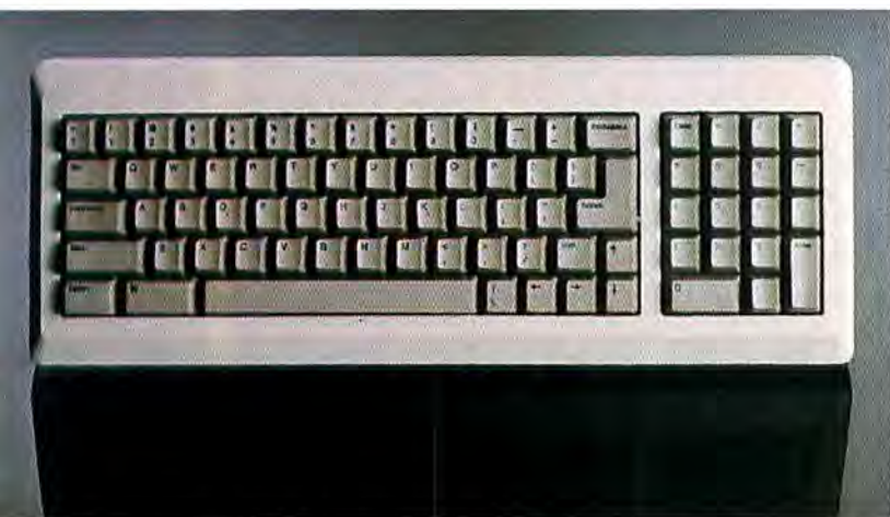
Figure 3 The arrow keys added to the right side of the Plus's keyboard result in a half-size right Shift key, which can be awkward to use at first.
