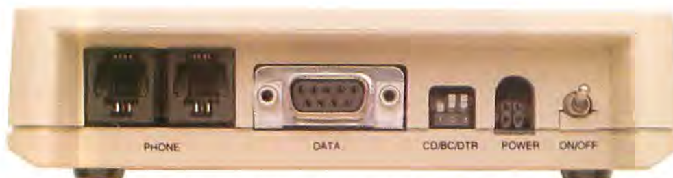
Sockets on the back of the Modem 1200 let you hook up to telephones and a telecommunications cable, and toggle switches enable you to configure various software and hardware combinations.
