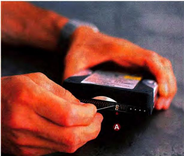
First, locate the small array of tiny pins on the side panel of your drive, between the ATA and power jacks. Some of the pins may already be connected to one another by one or more jumpers **A**.
