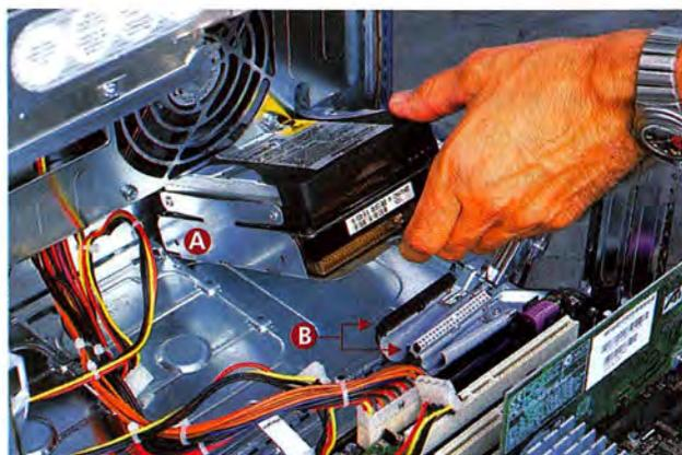
Slide the whole drive carrier into the computer case, lowering the back of the carrier in first **A**. Two metal tabs on the bottom of the carrier line up with slots in the bottom of the computer chassis. Slide the tabs into the slots, and then lower the front of the drive carrier into place. Attach it to the chassis using the Phillips screw you removed earlier.
