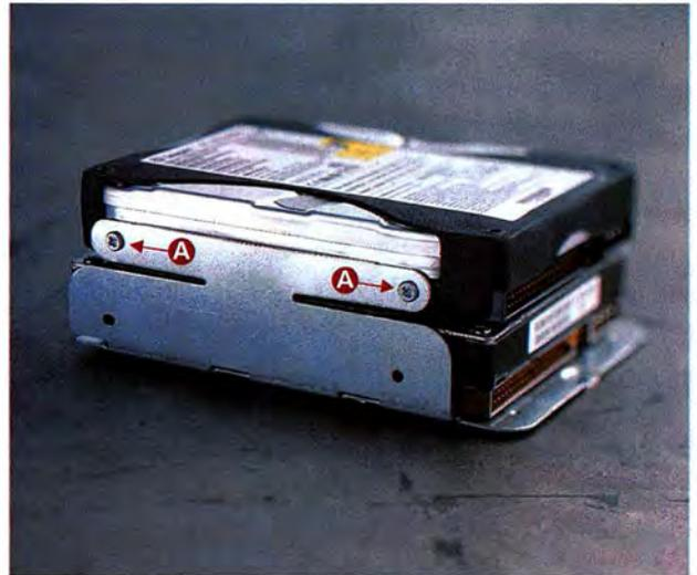
Slip the new drive into the upper portion of the carrier so that it piggybacks on the original drive. On the sides of the drive you'll see four screw holes that correspond to four holes **A** in the carrier itself. Use the screws that came with your drive to attach the drive to the carrier through these holes.
