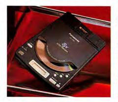
Portable, speaker-equipped CD-ROM drive is fast when plugged in but slow when on batteries.
