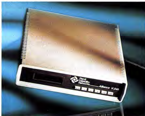
V.34 plus modems such as the Penril Alliance V.34bis (above) and others, from AT&T Paradyne, U.S. Robotics, and Motorola, can transfer data at a blistering 33,600 bits per second.
