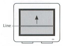
**Probable diagnosis:** Radio frequency interference (RFI) emanating from the Macintosh analog board (located on the left side of the Mac's cabinet) is causing the line.
