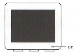
**Probable diagnosis:** The brightness and contrast controls (located on the right side of the cabinet) have been inadvertently turned down.
