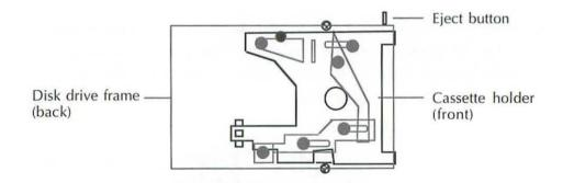
9. Carefully remove any dust, dried-up grease, etc. from the cassette holder assembly. Relubricate with WD-40 as necessary.
