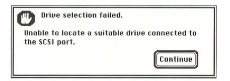
**Probable diagnosis:** The SCSI driver has been damaged or replaced by optimizer software, protection software or a generic SCSI utility.
