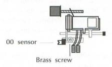
HEAV AUGWME 24. When the drive can initialize a disk, but can't read disks that you know are good, it means that the stepping motor assembly (consisting of the stator and the rotor) is out of alignment. Mark the original position of the stator assembly on the disk drive frame (draw
