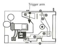
6. Using an ordinary pin, carefully release the cassette holder springs from the DD frame. There are two springs, one per side, located about halfway down each loading rail. Stretch/release only the bottom of the springs (not the tops).
