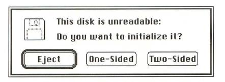
**Typical history:** The problem started right after a stuck disk was forcibly ejected from the drive (yanked out with pliers).
