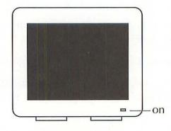
**Probable diagnosis:** The brightness and contrast controls (located on the right side of the cabinet) have been inadvertently turned down.
