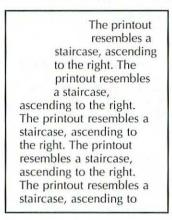
**Probable diagnosis:** There's too much friction on the carrier shaft and the carriage guide rail.
