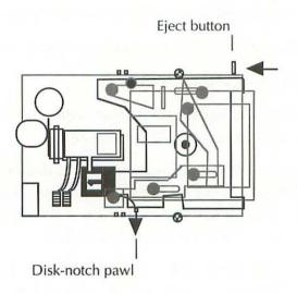
5. Lower the cassette holder assembly (to put it in "disk-in" mode) by engaging the trigger arm located on the right side of the cassette holder. Push gently in the direction indicated by the arrow.
