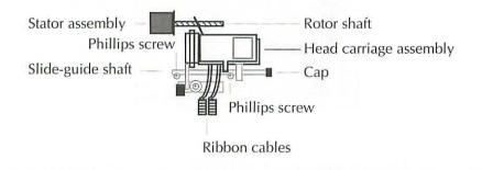
13. Slip the slide-guide shaft out of the old head carriage assembly. Slip the slide-guide shaft into the new head carriage assembly. Cap the slide-guide shaft, if necessary.
