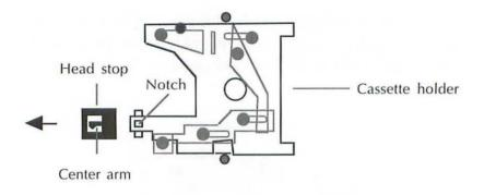
8. Remove the cassette holder from the disk drive frame. Lift up on the front of the assembly, then push the eject button about halfway in (if necessary), then lift up on the back of the assembly.
