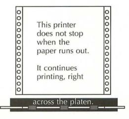
**Probable diagnosis:** The paper error detector is malfunctioning. Most likely, a mailing label got stuck under the platen and the detector arm is jammed by a piece that's still in there.
