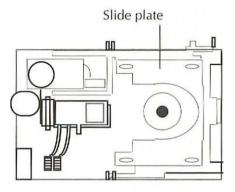
11. Examine the disk-notch pawl at the left-rear corner of the cassette holder assembly. Push the lever in the direction indicated by the arrow. Upon pushing the lever, the disk notch pawl will appear in the opening as shown. If necessary (because a disk was forcibly ejected with pliers and the pawl arm is horribly mangled), bend the pawl arm back into shape, then reinstall the cassette holder assembly and verify that the eject function works reliably.
