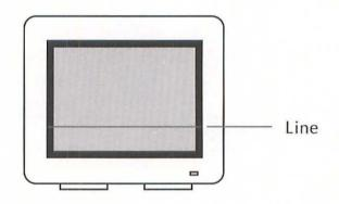
**Probable diagnosis:** The thin line is a characteristic of the particular Trinitron CRT (Sony part M34JNQ10X) used in this monitor. There's nothing to be done about it.
