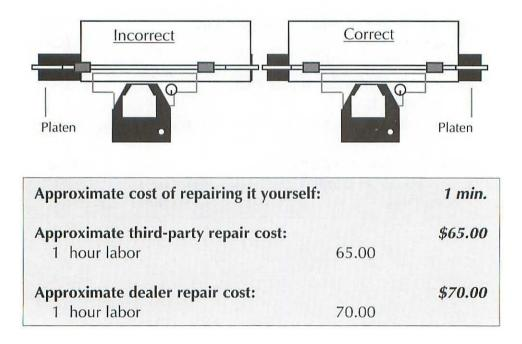
**Symptoms:** The ribbon carrier makes a scraping noise as it moves from side to side. Printed pages contain regularly spaced horizontal scratch marks (even in the white spaces).
