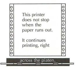
**Probable diagnosis:** The paper empty sensor is malfunctioning. Most likely, a mailing label is stuck under the platen.
