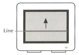
**Probable diagnosis:** Radio frequency interference (RFI) emanating from one or both of the monitors is causing the line(s).
