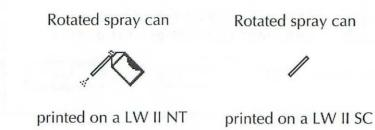
**Probable diagnosis:** Unlike the LaserWriter II NT and II NTX, the LaserWriter II SC doesn't have PostScript in ROM.
