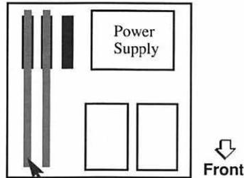
Configuration happens sequentially, beginning with the card in this slot
