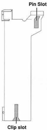
6. Remove the expansion cover shield which corresponds to the expansion slot you want to use for Spectrum/8 Series III. The cover shield is a bright metal bracket, and is located inside the main computer unit, along the back of the case. Lift the shield gently up and out of the computer, freeing it from the clip, and the pin that hold it in place. Save the shield; you will need to replace it if you remove Spectrum/8 Series III from it's slot.
