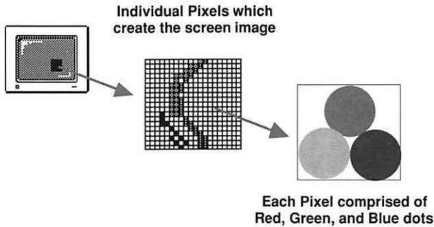
Deep inside the monitor are three separate electron “guns” which illuminate the red, green and blue color dots. Each gun only fires electrons at its corresponding color dots. These guns can vary in intensity: if more electrons are directed at a particular color dot in a pixel, that color dot glows more brightly.
