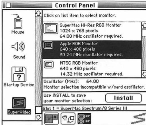
For complete information about using the Monitor Configuration Utility, refer to the owner's manual which was supplied with your SuperMac Spectrum video card.
