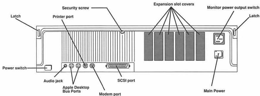
2. Using a Phillips screwdriver, loosen and remove the security screw from the back of the Macintosh II case.
