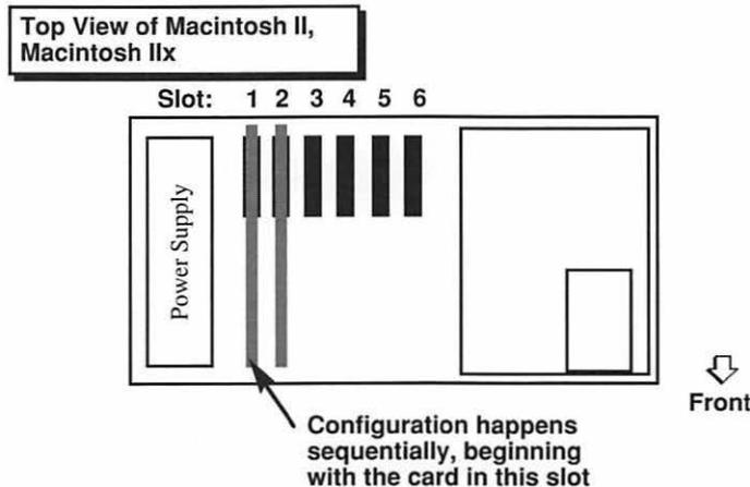
For the Macintosh IIcx and IIci, this is the NuBus slot which is *farthest* from the power supply, as illustrated by the diagram on the next page:
