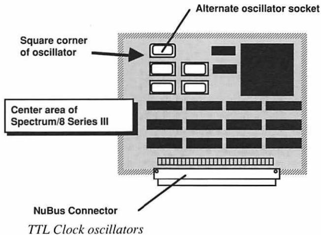
4. The empty socket is the one nearest the top of the video card. Align the TTL Clock Oscillator over this socket so that the square corner of the oscillator is pointing toward the NuBus connector, and the four pins are over the four "holes" in the empty socket on the Spectrum/8 Series III.
