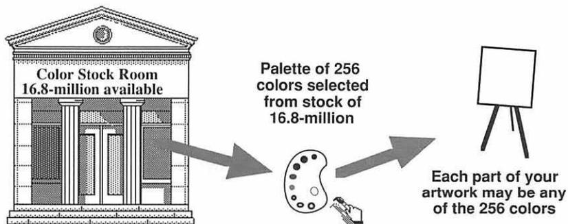
This is exactly how an 8-bit Macintosh video system works. Of course, instead of dabbing paint on a canvas, the colors are defined electronically. From the 16.8-million color possibilities, 256 colors are chosen to be on the screen at any one time, and each pixel on the screen can be any of the 256 colors. When the Macintosh calls for a specific
