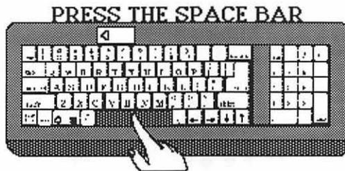
4. When this screen appears, *immediately* press the space bar on the keyboard, and the Macintosh will restart to lock-in in the configuration.
