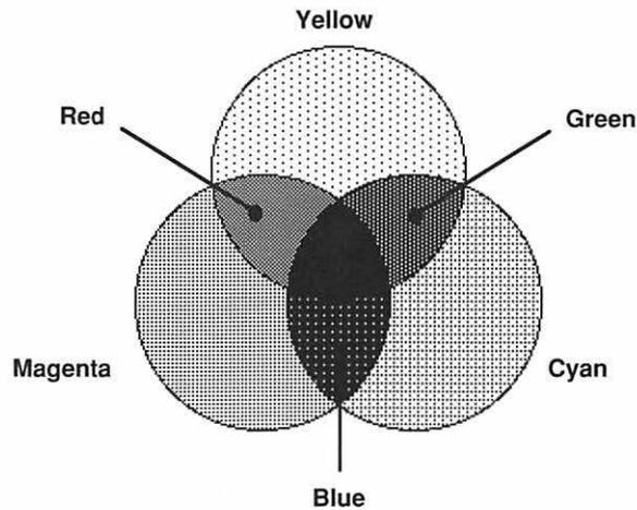
Note that the center of this diagram, where all three colors overlap in equal amounts, the result is black. In other words, the three Subtractive Primaries work together to *subtract* all colors of light — and the result is the absence of light. Pure black.
