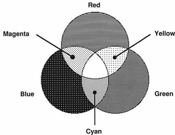
Notice that the center of the diagram, where all three colors overlap in equal amounts, the result is white light.
