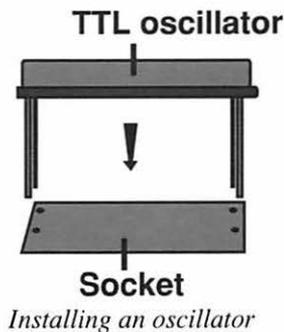
5. Gently push the TTL Clock Oscillator into the socket, making sure that all four pins are guided straight into the holes of the socket.
