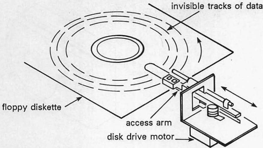
Fig. 5-8. Floppy disk drive diagram.
