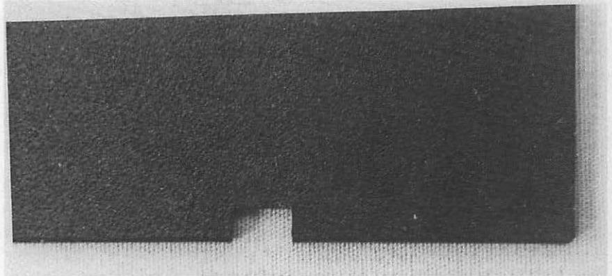
Fig. 5-10. 5¼-inch diskette write-protect notch.
