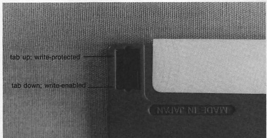
Fig. 5-11. 3½-inch diskette write-protect notch.
