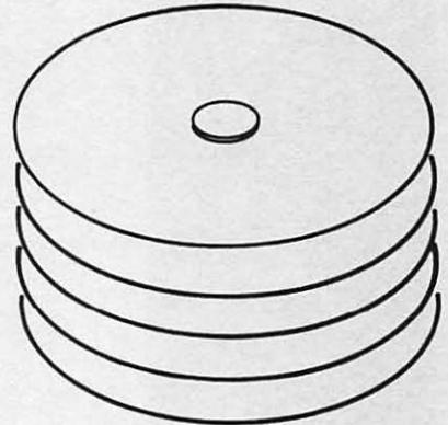
Fig. 5-3. Fourteen-inch mass storage platters.
