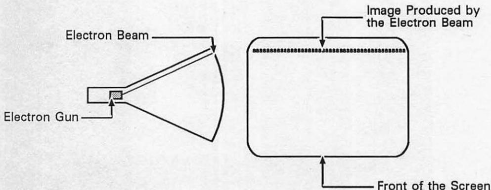
Fig. 3-4. Monitor and electron beam.
