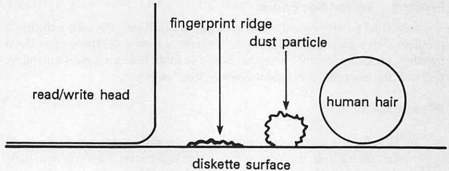
Fig. 5-16. Disk contamination.
