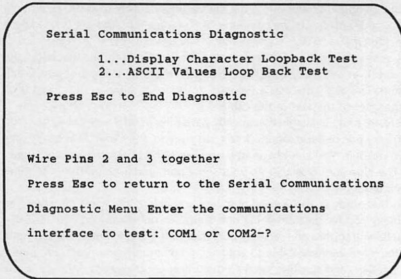
Fig. 6-9. Serial communications test instructions.
