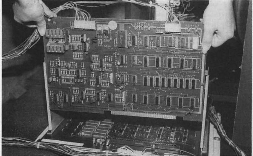
Fig. 1-11. Removing the board from its slot.
