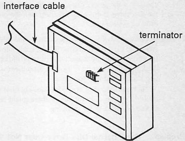
Fig. 5-15. Terminator strip in daisy chain port.
