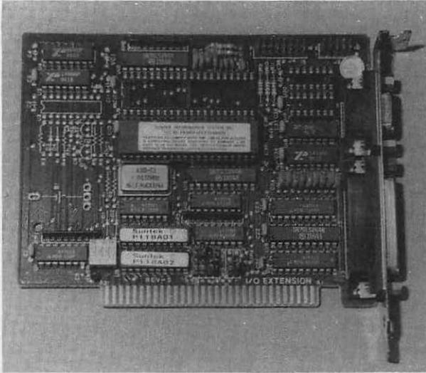
Fig. 6-1. Serial communication interface board.
