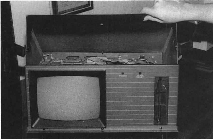
Fig. 1-10. Opening the system unit.
