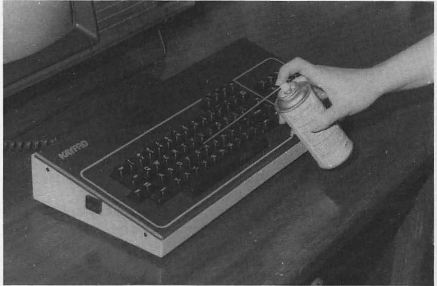
Fig. 1-8. Dusting with compressed air.
