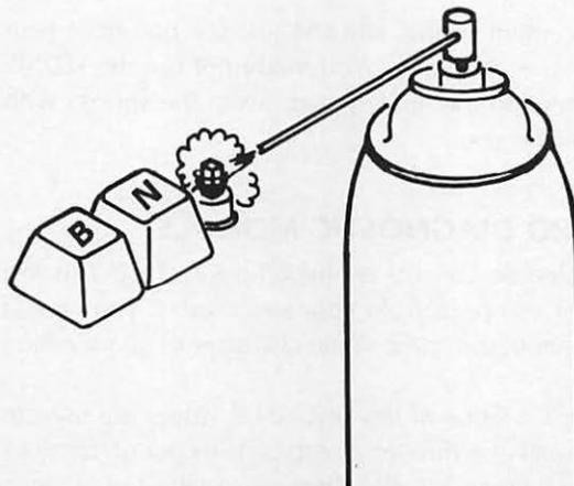
Fig. 2-6. Spraying contact cleaner on key post.
