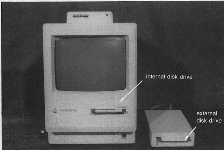
Fig. 5-2. Internal and external disk drives.
