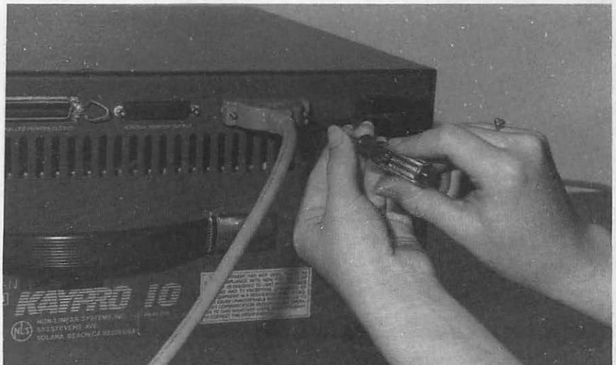
Fig. 1-9. Tightening cable screws.
