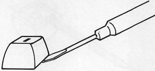
Fig. 2-5. Lifting key from key post.
