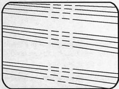
Fig. 3-6. High brightness lines on monitor.
