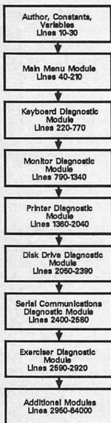
Fig. 1-2. Diagnostic program block diagram.
