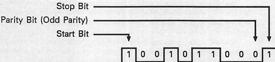
Fig. 6-5. Start bit and stop bit.
