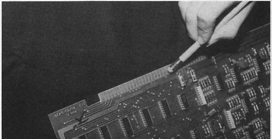
Fig. 1-12. Erasing oxidation from the edge connector.
