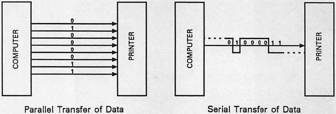
Fig. 4-5. Parallel and serial data transfer.
