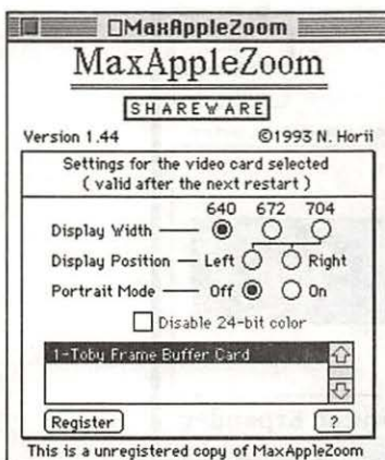
Figure 9.22 Setting monitor resolution with MaxAppleZoom
