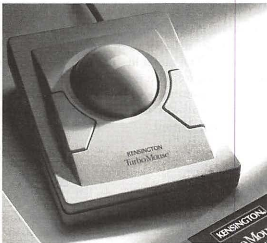
Figure 9.3 A trackball (the Kensington TurboMouse)
