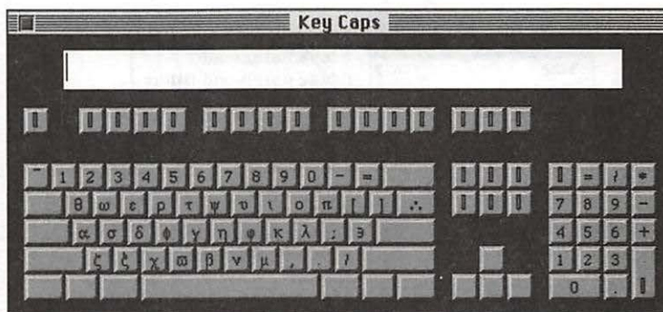
Figure 4.13 Using Key Caps to see the characters generated by specific key presses
