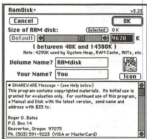
Figure 6.7 Setting the size of a RamDisk+ RAM disk
