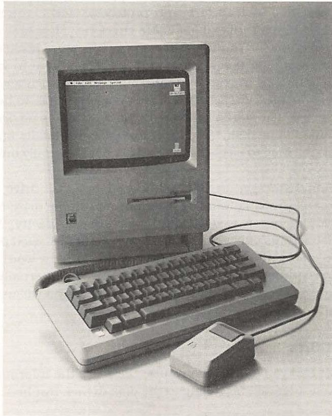
**Fig. 1-2** Macintosh has a 9-inch screen, an integral microfloppy disk drive that takes 3½ inch disks, a detachable keyboard, and a mouse input device.
