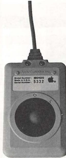
**Fig. 3-4** At the bottom of the mouse is a ball that rides freely along the surface of a desk.
