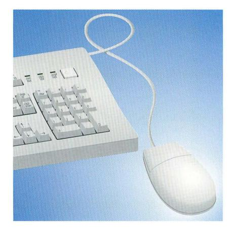
**BECAUSE** they are the primary data-entry and control devices, the keyboard and the mouse are the peripherals you spend the most time with. Since the introduction of the Mac SE in 1987, all Macs have used the Apple desktop bus, or *ADB*, to connect the computer to the mouse and keyboard. The built-in trackballs and trackpads in PowerBook laptops also use ADB. Some Macs have a single ADB port, though most models have two.
