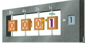
2 To increase the number by 1, we spin the 1's place sign again, returning it to 0. This causes the lever to flip the sign in the 2's place from 0 to 1. We start with 0000 and rotate the sign in the 1's place from 0 to 1. The lever hits the sign on the next column and stops.
