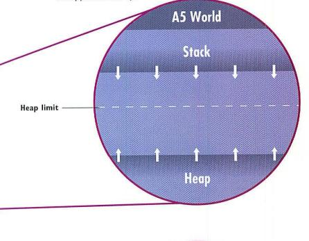
Most of the action occurs in the application *stack*, which holds temporary values, and in the application *heap*, which holds code segments, resources, and document data. The stack and the heap are dynamically allocated, constantly expanding into and retreating from an empty area of unallocated memory that sits between the two. The application stack can temporarily fill the entire unallocated space, but the heap can fill only a portion of it.
