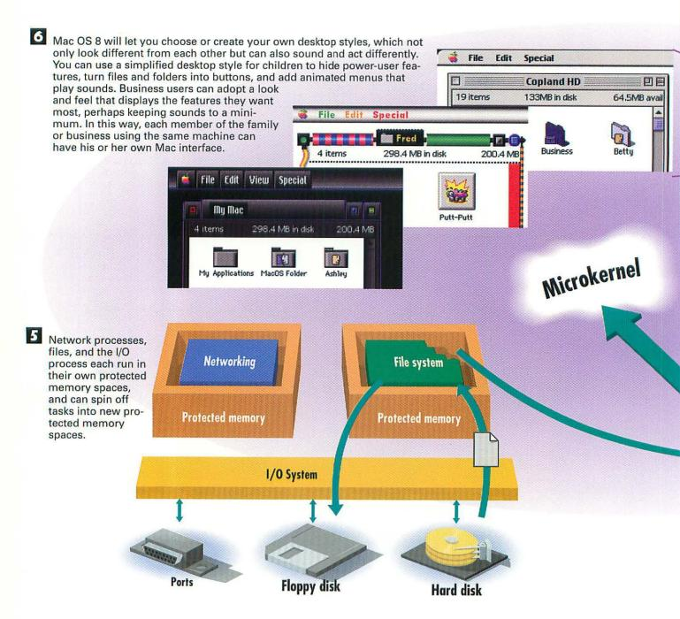
2 Preemptive multitasking is a new feature that lets the Mac do several tasks at once. The code for each task runs in a completely separate, protected memory space. This will let you save a document to a floppy disk at the same time you type in a word processor. If the software in one protected memory space crashes, it won't affect the rest of the Mac, and you won't have to restart your computer.
