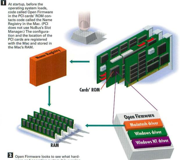
Open Firmware looks to see what hardware and operating system it is running in. It then loads the Mac driver into RAM. On a Windows machine, the same card would load a Windows driver into the PC's RAM. Open Firmware is an industry standard, IEEE 1275.
