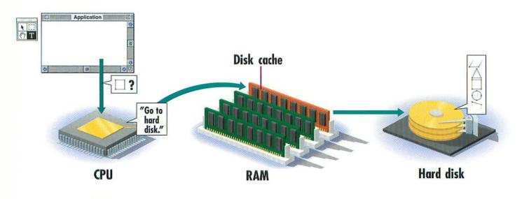
Mac OS sets aside at least 32K of RAM to be used as a disk cache, although the user can enlarge this. This space is not available to be used as main memory. When an application makes a request for information that is residing on a hard disk, the disk cache intercepts the request and searches itself for the information. If it does not have the requested information, it passes the query along to the disk.
