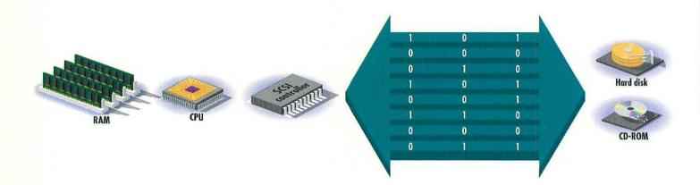
**Ordinary SCSI** SCSI transmits bits of information in a parallel fashion, moving groups of 8 bits (called a byte) between the Mac's RAM and storage drives. The SCSI controllers in the Mac and the disk drives can put a maximum of 5 million of these bytes (5MB) on the SCSI bus every second.
