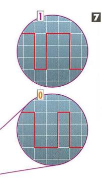
A data bit is sent as a low voltage followed by a high voltage. A 0 is represented by a long low voltage (65 microseconds) followed by a short high voltage. A 1 is represented by a short low voltage (35 microseconds) followed by a long high voltage. Commands also use this scheme, varying the lengths of the voltages in different ways.
