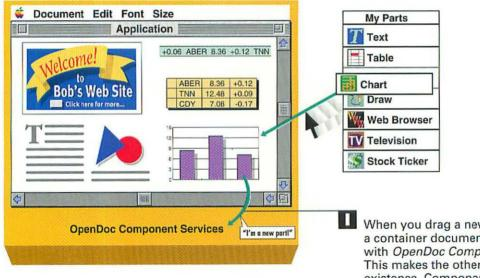
When you drag a new OpenDoc part into a container document, it registers itself with *OpenDoc Component Services*. This makes the other parts aware of its existence. Component Services allows parts to work together, sharing code and other resources.
