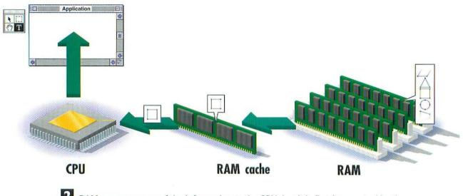
**2** RAM passes a copy of the information to the CPU, but it is first intercepted by the cache. The cache makes and keeps a copy, and passes a copy to the CPU.
