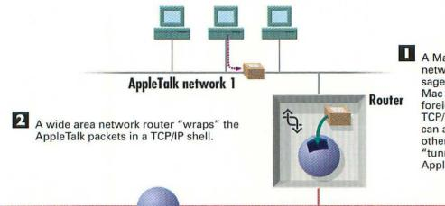
A Mac on an AppleTalk network sends out a message that is addressed to a Mac on the other side of a foreign network, such as a TCP/IP network. The user can access a Mac on the other side of the AppleTalk "tunnel" by using ordinary AppleTalk software.
