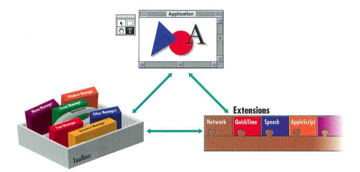
**EXAMPLE** System extensions sometimes follow a migratory path, starting as an add-on extension, then later being included as a built-in part of the system software, and finally becoming an actual Toolbox routine in ROM. 32-bit color QuickDraw, which started out as an extension, was included in the Mac ROM starting with the Mac IIci.
