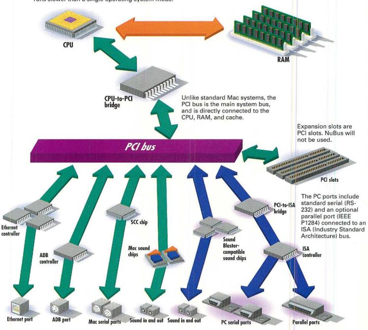
The Mac ports include an Apple desktop bus (ADB) for keyboard and mouse, and printer and modem ports enabled for LocalTalk and GeoPort.
