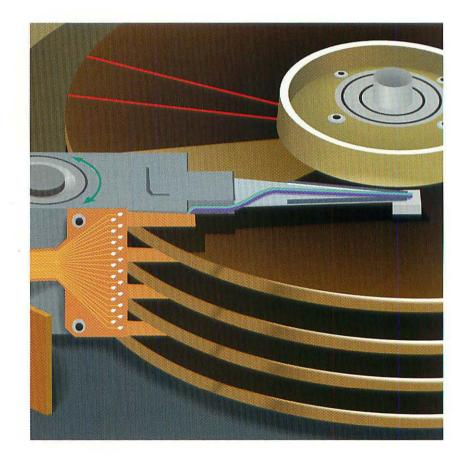
hard-disk drive is the method of data storage most Mac and PC users continually depend upon to hold and retrieve software and the work we produce. A highprecision machine, the hard-disk drive is the fastest mechanical storage device available, second only to RAM (which is nonmechanical) in speed, but far less expensive.
