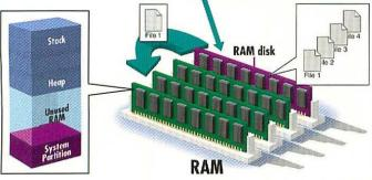
Double-clicking on a file in a RAM disk loads the file from the RAM-disk portion into real RAM. The RAM disk stores the file as a document, just as disk drives do, rather than in the stack/heap format of an application's partition in main memory.
