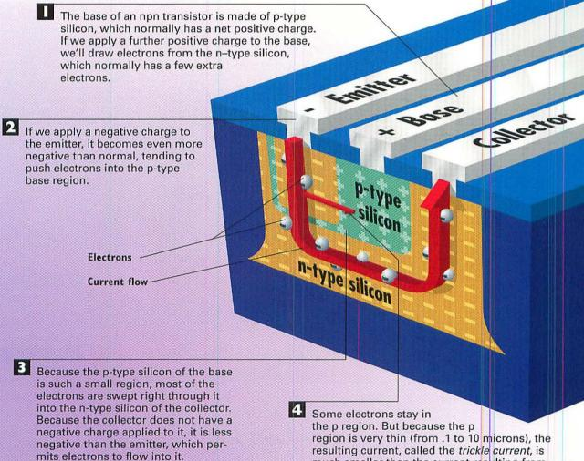
region is very thin (from .1 to 10 microns), the resulting current, called the *trickle current*, is much smaller than the current resulting from the electron flow from emitter to collector. In effect, the small trickle current controls the much larger current passing through the base from emitter to collector. 62 PART 3 CPU AND MEMORY
