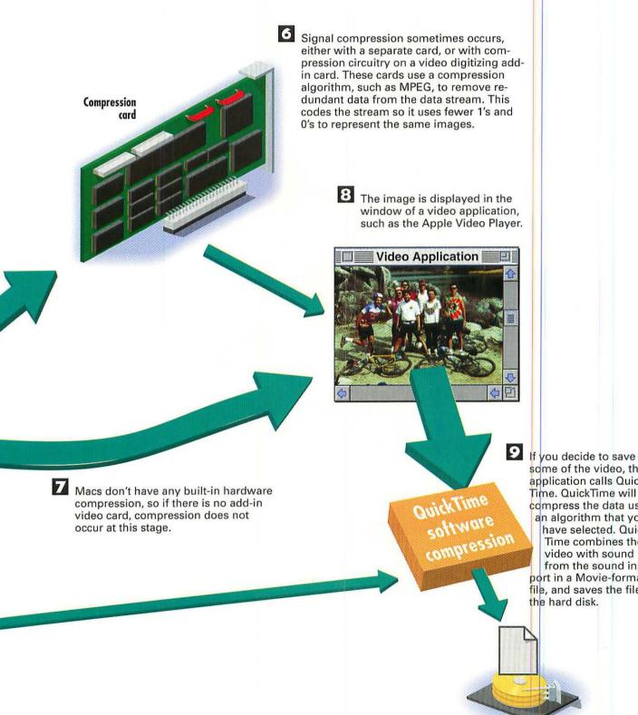
some of the video, the application calls Quick-Time. QuickTime will compress the data using an algorithm that you have selected. Quick-Time combines the video with sound from the sound input port in a Movie-format file, and saves the file to the hard disk.
