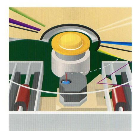
*can* take it with you. Replace the hard drive's multiple platters with a single disk, put it in a removable cartridge, and you have mass storage with the convenience of a floppy disk. Magnetic removable cartridges come in several formats, holding from 44MB to 1GB. The most popular ones use 3½-inch disks just slightly bigger than a floppy.
