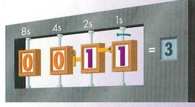
Adding another 1 to the 1's place causes the signs in both the 2's and 4's places to turn, giving us the binary number 0100, or decimal 4. 3 Increasing the number by 1 again causes the 1's place to advance from 0 to 1, but doesn't affect the 2's place.
