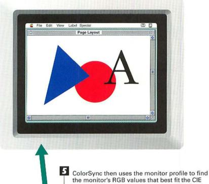
ColorSync then uses the monitor profile to find the monitor's RGB values that best fit the CIE values. Corrections can be made at this time to compensate for any nonuniform display characteristics of the particular monitor.
