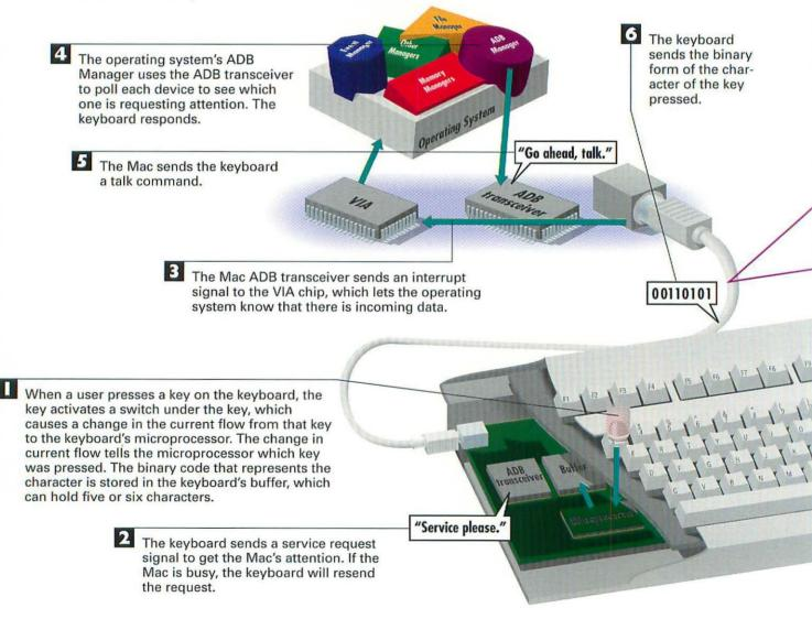
B The ADB transceiver in the Mac receives the keypress and passes it to the VIA, which sends a message to the operating system's Event Manager. This message is then passed on to the Toolbox Event Manager. Finally, the key is displayed on screen as a character or, if the user pressed a key
