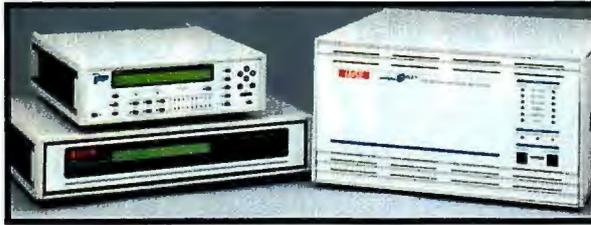
TAS Series II telephone network emulator and Model 240 loop emulator from Telecom Analysis Systems.
